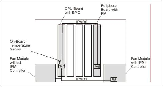
The devices are connected to the IPMB1 via the Intel<sup>®</sup> NetStructure<sup>™</sup> MPRTM4848 Rear Transition Board for the respective CPU board. The IPMB1 signals are routed from the IPMI controller on the CPU board to the RTB via the backplane and are then available at an IPMB1 connector of the RTB. This IPMB1 connector is located on-board the RTBs.
